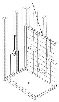
Drill plumbing holes in side wall panel; then proceed to side wall installation. (Step 5 on page 4)
