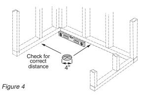
DRY-FIT SHOWER: Set shower pan in the pocket. You MUST use a level to ensure the unit is level. Shim if necessary.
