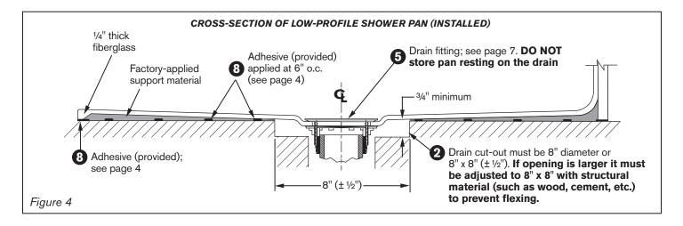
1 Check shower pocket area for level and for correct dimensions. Make sure drain hole in floor is the correct distance from studs. The floor must be within 1/6" of level, especially around drain box-out.
